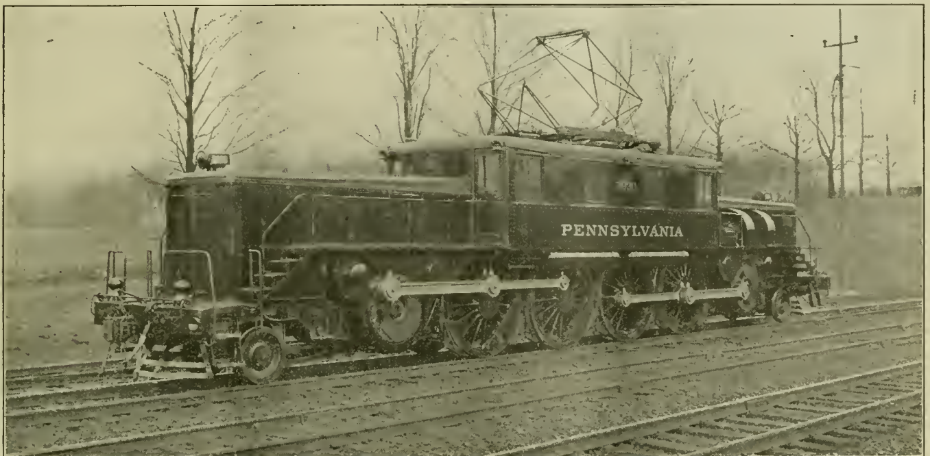
Pennsylvania Railroad's Class L-5 Electric Locomotive—Built at Altoona Shops of the Railroad Company
